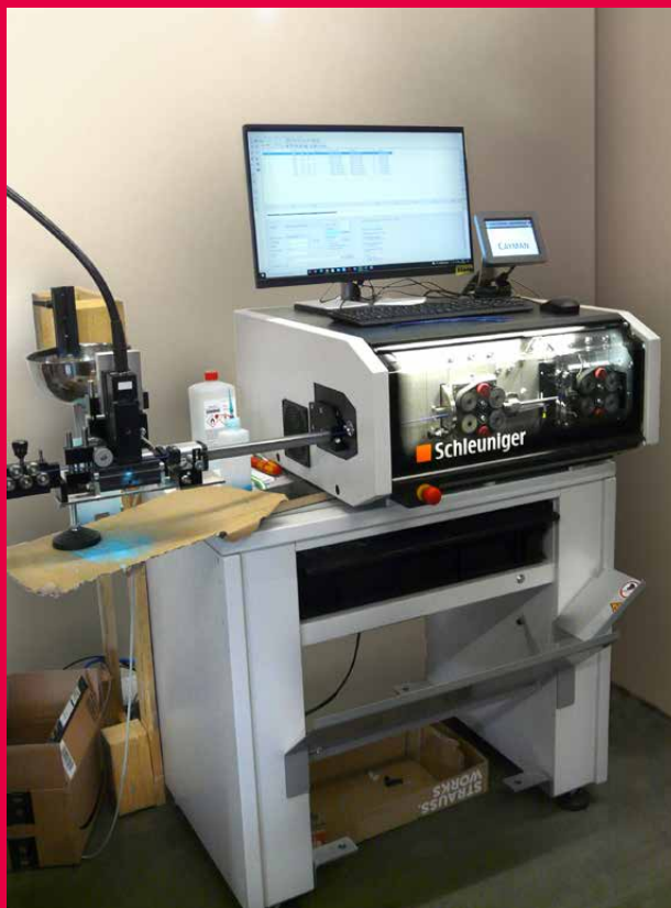
The new individual wire assembly and labelling system pulls its data from EPLAN Pro Panel.
